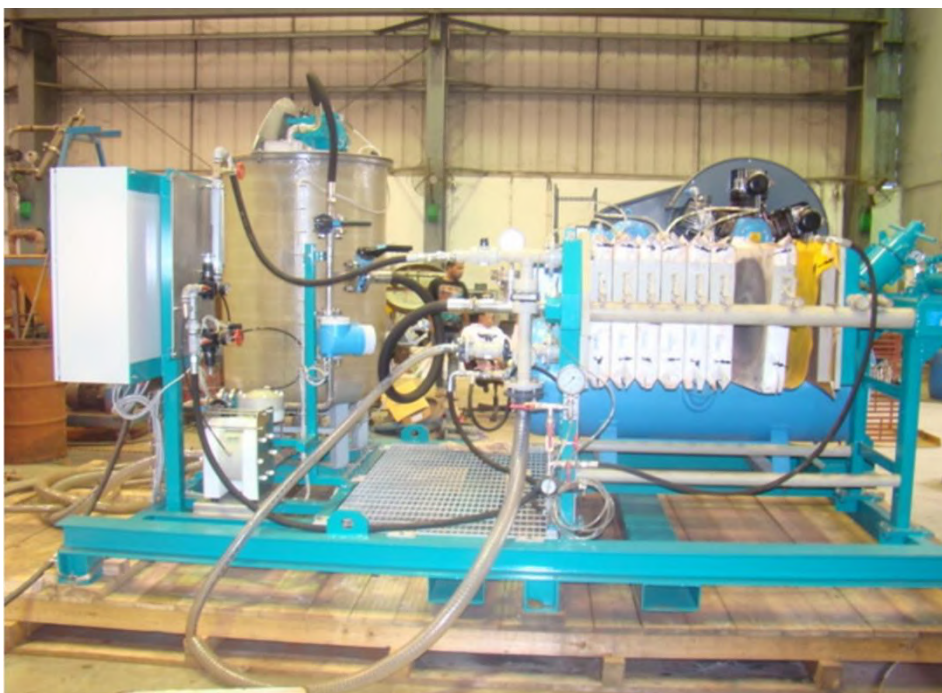
Fig. 3.8 Pilot scale pressure filter set up
