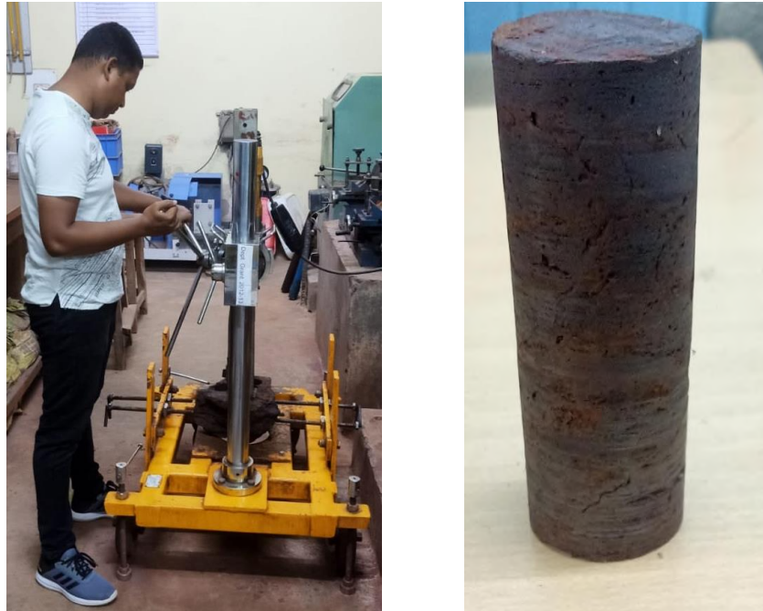
Figure IV. Coring operation and cored specimen
