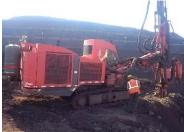
Wet Drilling And Dust Extractor System In Drilling Operation
