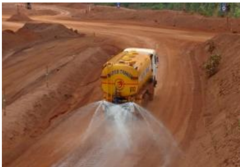
Water Tanker Arrangement For Haul Road Dust Suppression
