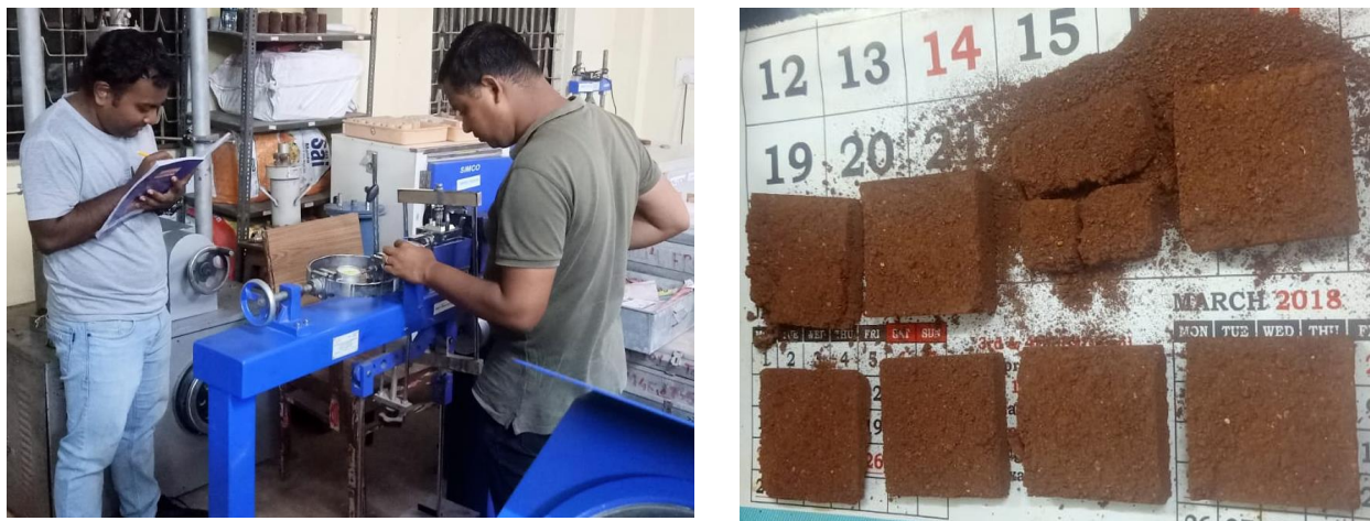
Fig VII: Direct Shear test
