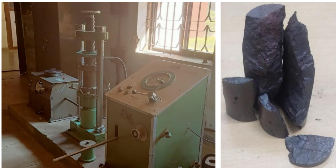
Fig VI: Triaxial Setup and Fractured Sample
