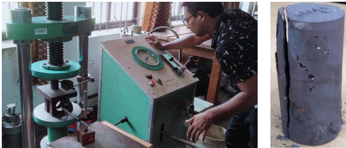
Figure V. Determining UCS of rock sample
